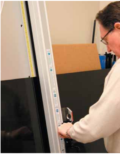
The Fletcher-Terry FSC cutting machine is designed for heavy duty applications, including ACM cutting and V-grooving.
