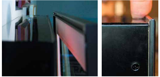
This end view shows how the lip of the inner frame extends past the perimeter of the ACM shadowbox to hold the face frame in place. (Detail) The standard-profile aluminum sectional face frame fits snugly over the inner frame's lip.
