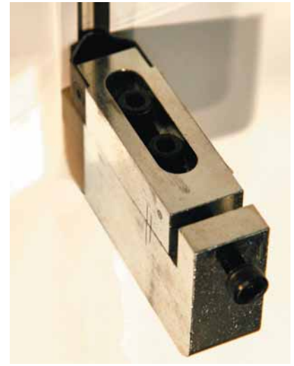
The V-grooving tool fits into the FSC machine's holder and cuts neat, 1/4" wide V-grooves in ACM up to 4 mm thick.
