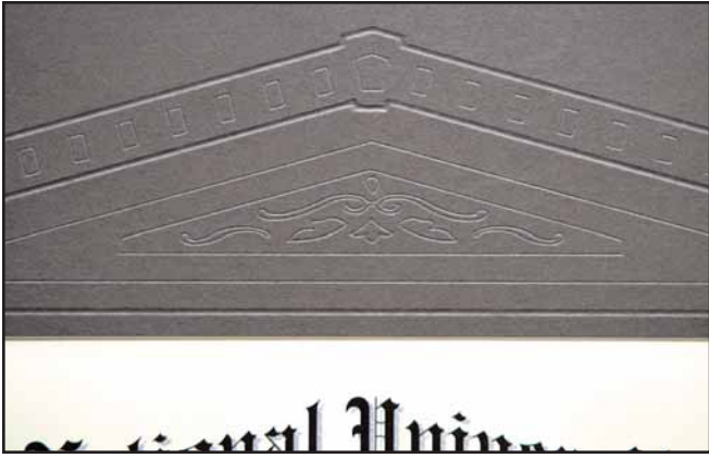
For a subtle decorative effect, the single operation of debossing shows the design only as shadows. If your CMC accessories include fine, medium, and wide debossing tips, use them in different combinations to emphasize certain parts of the design.
