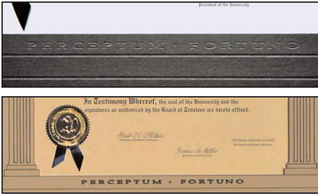
Fine details that do not cut or V-groove well, such as text smaller than about 1", look better debossed or inked. The text here is about 1/4" tall. It can be easily changed or removed from the design.
