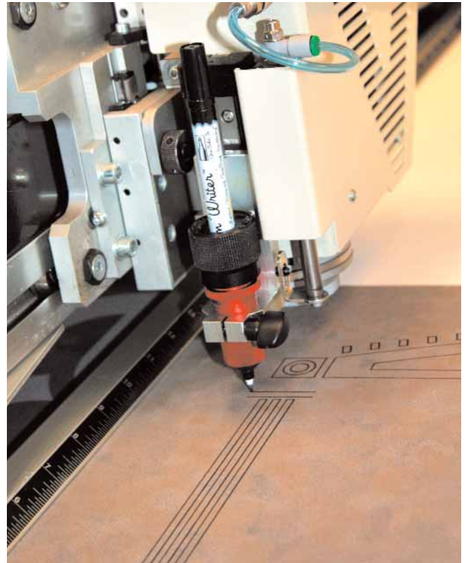
Standard ink pens can be used in the drawing attachments on CMCs. This technology is very useful in creative matting.
