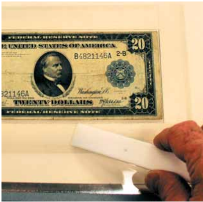
The final step of encapsulating each bill was to burnish the double-sided tape's adhesive.
