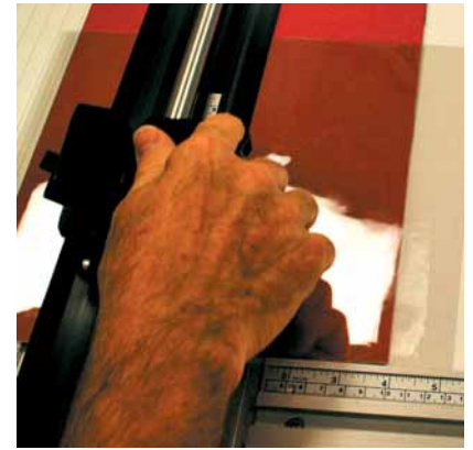
Melinex 516 clear polyester film was trimmed from a roll using the manual mat cutter. This machine enables the clear film pieces to be measured and cut quickly and precisely.
