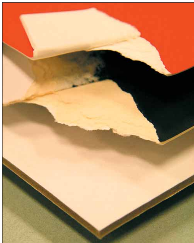
Paperboard substrates (top-to-bottom): preservation (alphacellulose) 4-ply matboard, non-preservation (acid-free) matboard, and Upson board.
