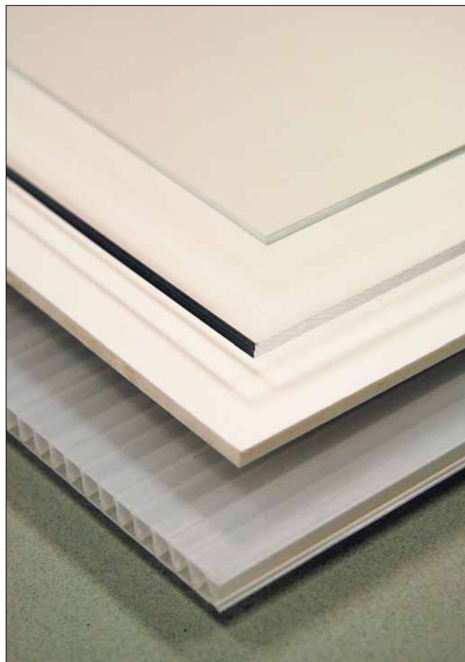
Plastic substrates (top-to-bottom): acrylic sheet (available clear or colored), polycarbonate, polyvinyl chloride (PVC), and fluted polypropylene.
