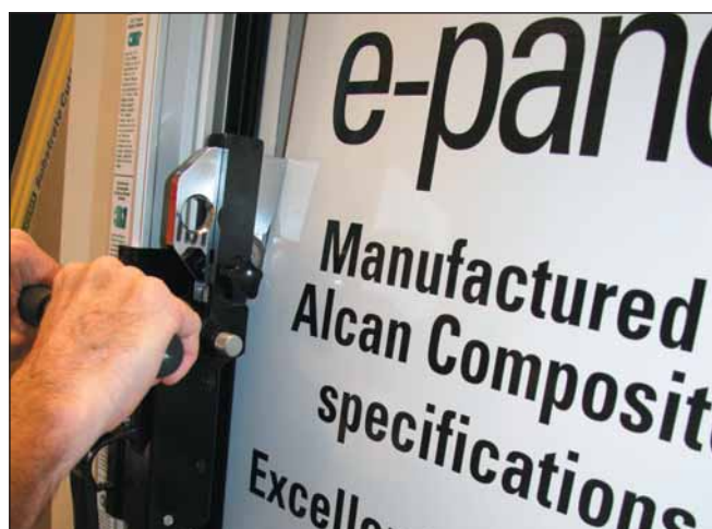
Aluminum composite material up to 4mm thick may be most neatly cut using a roller-type cutter, such as this attachment to the Fletcher FSC machine, to provide a smooth, rolled edge. A saw can also cut this material, but the edges would require finishing.
