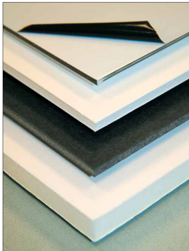
Composite substrates (top-to-bottom): aluminum composite material (ACM), white foamboard, black foamboard, and high-density foamboard.
