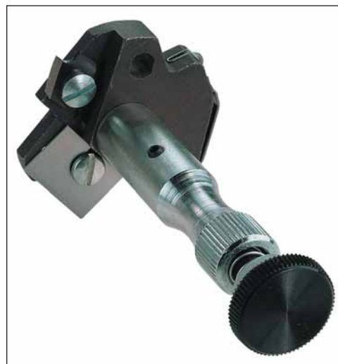
A convenient turret holds all three cutting tools used with a wall-mounted cutter—a glass cutter, an acrylic cutter, and a knife for paperboard.
