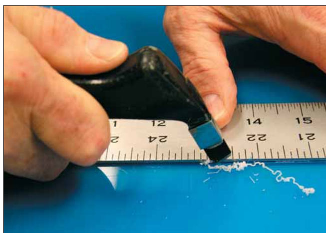
An acrylic sheet can be cut using a hand-held tool and straight edge, as shown here, but an acrylic cutting attachment in a wall-mounted machine is more convenient for the purpose.
