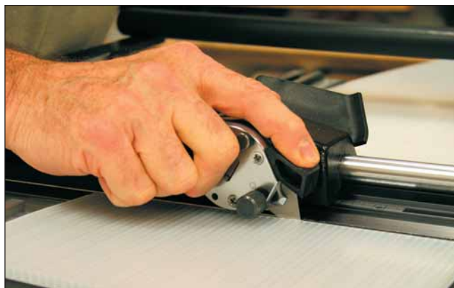
Fluted polypropylene may be cut using a machine-mounted blade, such as this mat cutter or a wall-mounted cutter. A hand-held knife and straight edge can also do the job.
