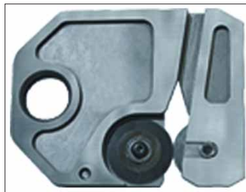
Aluminum sheets can be cut using roller-type cutters, such as this one for a wall-mounted cutter.
