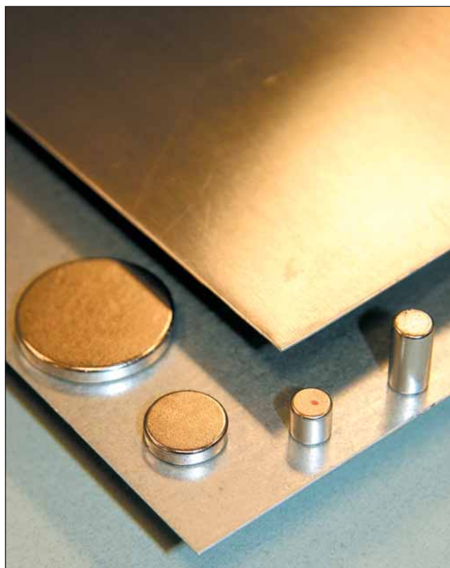
Metal substrates (top-to-bottom): unfinished aluminum sheet and unfinished steel sheet. In certain mounting applications, rare-earth magnets may be used, such as the ones shown here.
