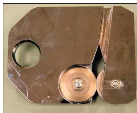
Robust roller-type attachments like this are used to cut aluminum composite material up to 4mm thick.
