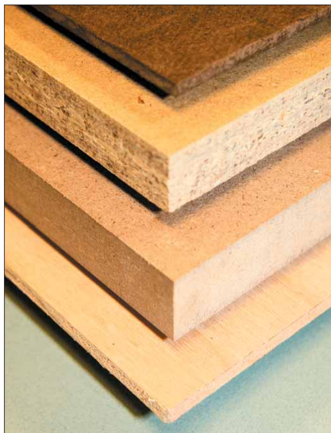
Wood product substrates (top-to-bottom): hardboard, particle board, medium density fiberboard (MDF), and plywood.
