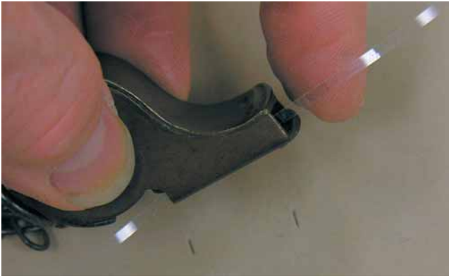
One clear film strap, about \frac{1}{8} " wide, holds the whistle securely in place.
