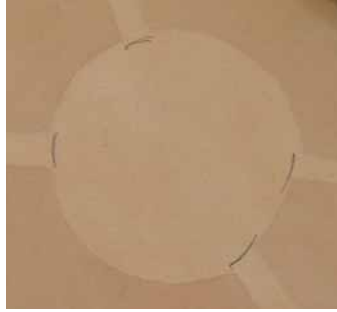
The scrap from the template was used to mark slot locations with light pencil lines on the mount board. Note that the slots are placed slightly inside the perimeter of the compass so they will be covered when the mount is completed. Then the mount "legs" were pulled through the slots.
